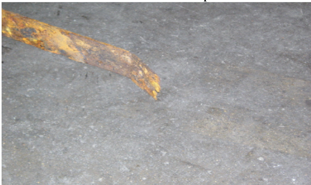
Failed Fuel Tank Strap
