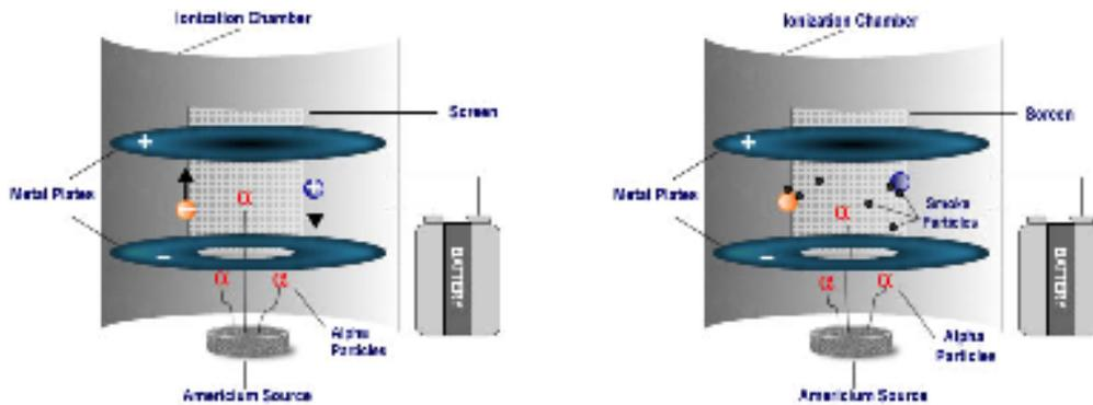
Smoke particles and combustion gases interact with the ions generated by the alpha particles, restoring them to their neutral electronic state and decreasing the electrical current passing through the cell.
