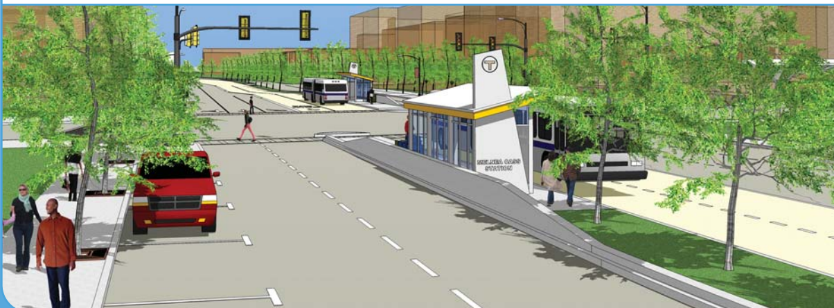
The rendering depicts a center median busway with landscaping on Melnea Cass Boulevard.
