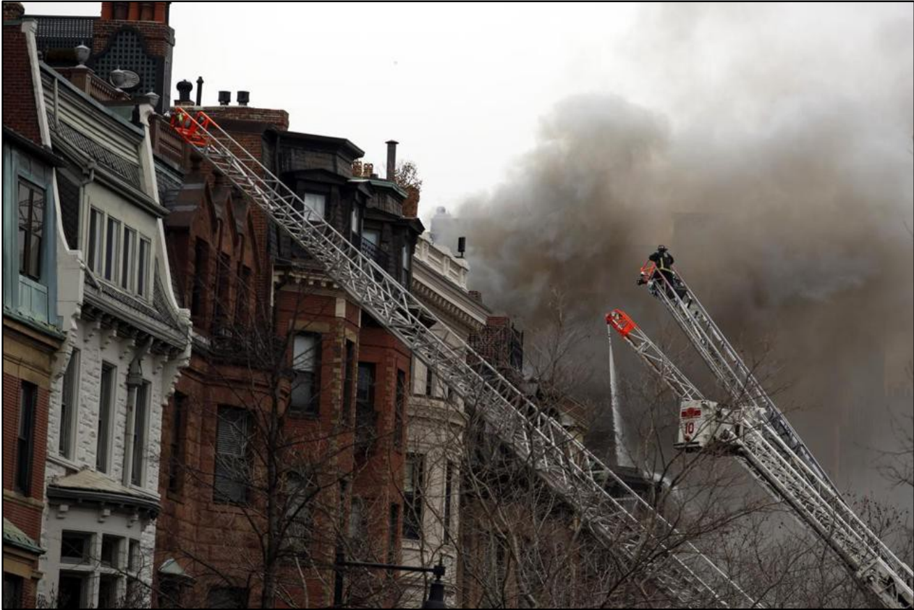
Photo 4. Defensive operations on Side Alpha of the fire building. Three ladder pipes, a tower ladder, numerous deck guns, and hoselines are in operation. The time is approximately 1615 hours. (Photo courtesy of the fire department.)
