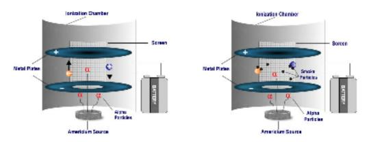
Smoke particles and combustion gases interact with the ions generated by the alpha particles, restoring them to their neutral electronic state and decreasing the electrical current passing through the cell.
